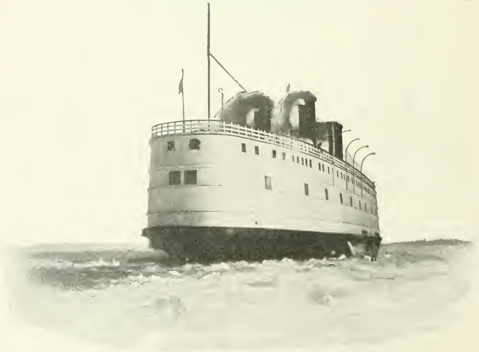
ICE-BREAKING TRAIN-FERRY BAIKAL Carrying trains of the Trans-Siberian Railway across Lake Baikal
